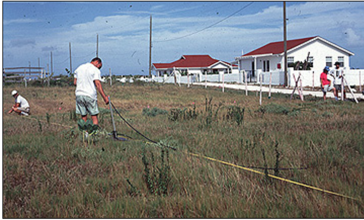
Ground penetrating radar survey of GT-3. Photo © Betsy Carlson)
