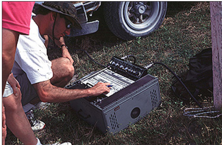
GPR printout of radar hits on buried features. (Photo © Betsy Carlson)
