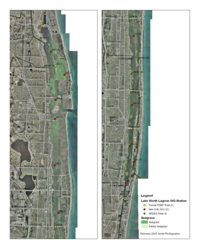
Figure 31. Water quality monitoring stations at the Lake Worth Lagoon and three canals discharging freshwater to the system. Six stations were sampled from 2001-2005 (yellow circles) and eighteen (18) stations were sampled from 2007-2012 (yellow and red circles).
