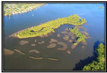
open space provides an edge between the sand and rock, allowing fish and invertebrates easy entry to the rock structures and water flow. Water flow is important to oyster health by delivering oxygen and food, and for settlement of oyster spat. Project partners included the Town of Palm Beach and Florida Inland Navigation District. Just north of the Ibis Isle Restoration Project, this site is also known for foraging American oystercatchers and osprey.
