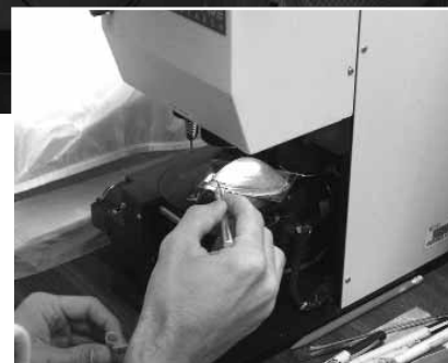
Close-up of the microdrill being used by Matt to collect minute samples from individual growth rings of surf clams from the Useppa Island midden. Here Matt uses an Exacto knife to collect the material he has just drilled. (Photo by W. Marquardt.)
