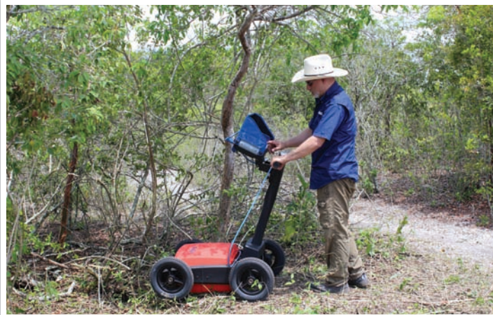
Victor Thompson operates the GPR on Mound 1.
