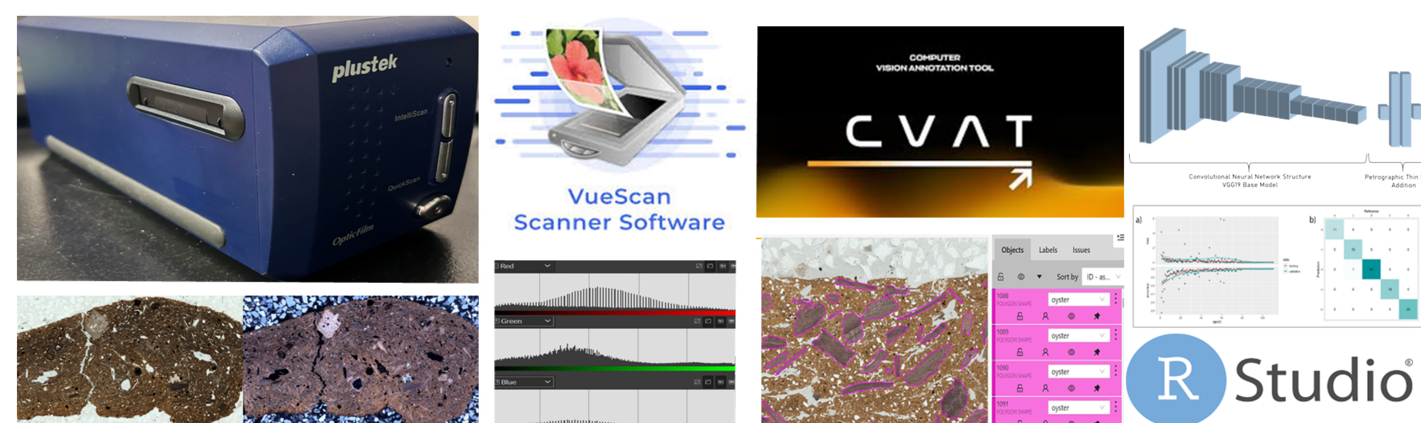
Figure 3. Using a low cost film scanner (PlusTek 8100 OpticFilm scanner), 3D-printed slide holders, and polarizing filters, thin sections can be scanned in plane and circularly polarized light. VueScan is then used to process and edit these scans, and inclusions and voids of interest can be annotated in CVAT. These annotations can then be used to train a CNN model in R or Python [4].
