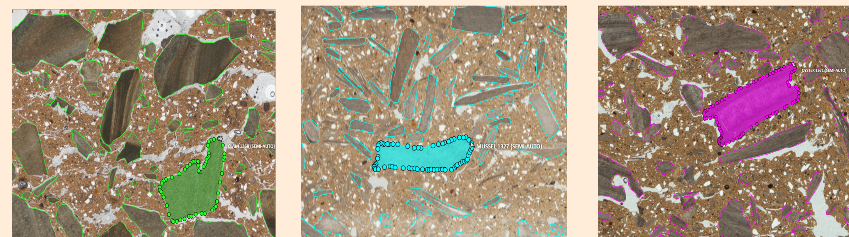
Figure 4. Experimental thin section samples with known inclusion types and frequencies. Clam shell in green, Mussel Shell in blue, and Oyster in pink.
