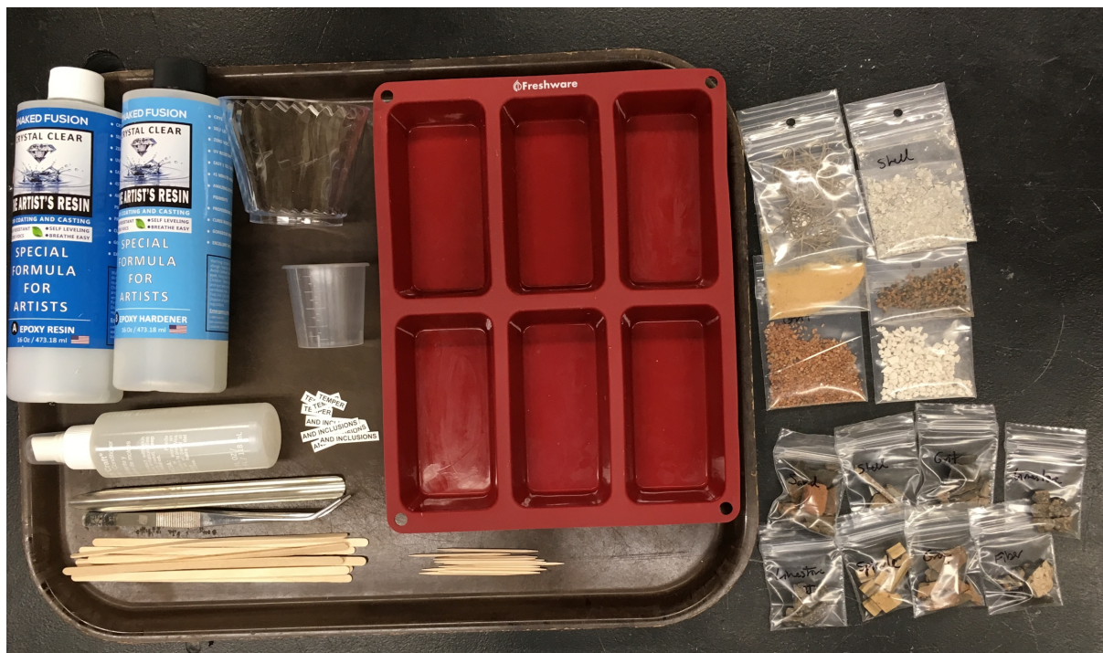
Figure 1. Materials for preparing blocks. Clockwise from top left: liquid resin part A and B, resin mixing and measuring cups, silicone mold, bagged inclusions, sample sherd slices, toothpicks and stirrers, cardstock labels, tweezers, sample spoon, mold release agent.
